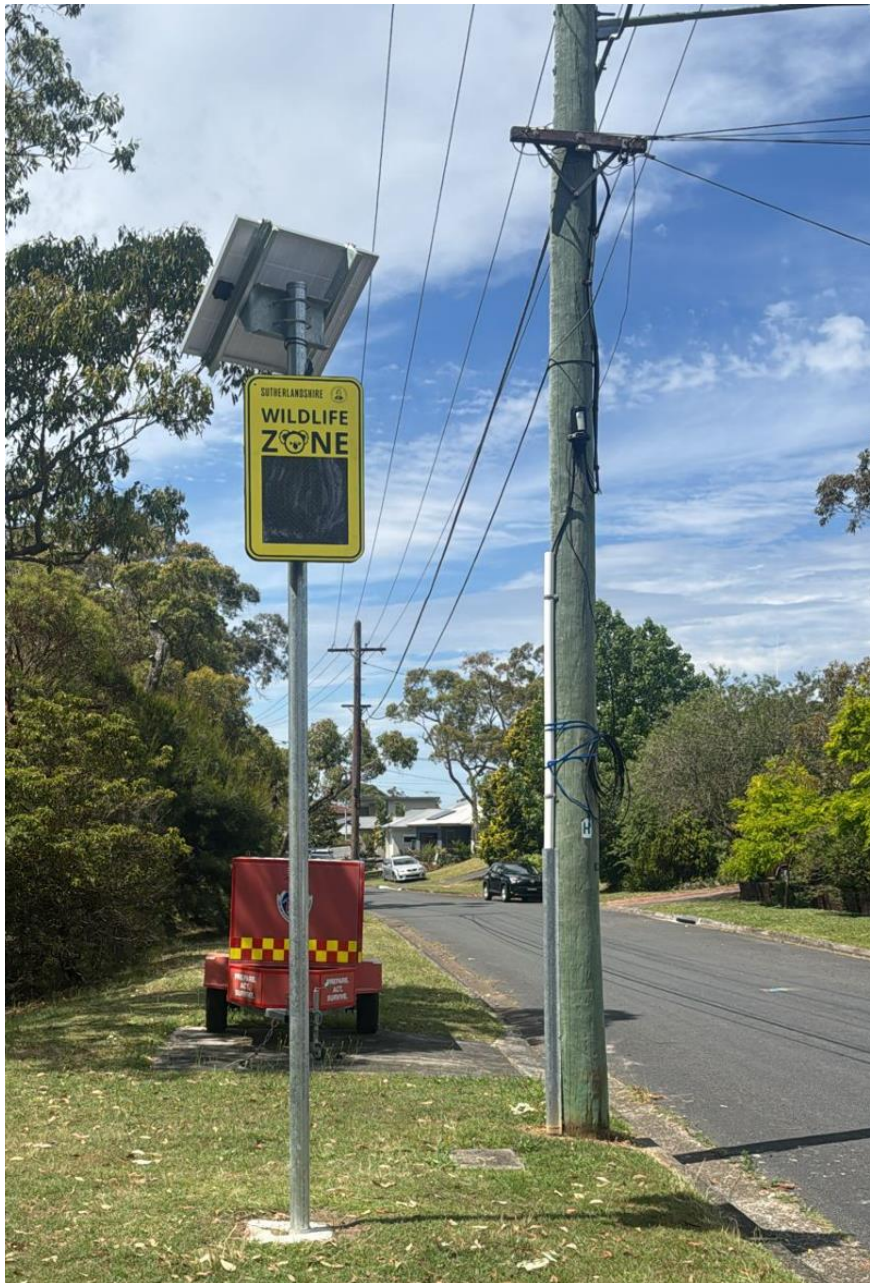
Figure 14 Example of a vehicle activated sign installed by Sutherland Shire
