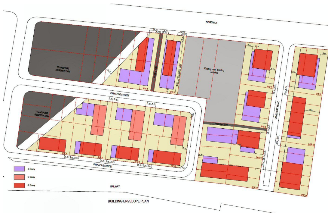
Miranda Pinnacle Street Precinct Building Envelope Plan
