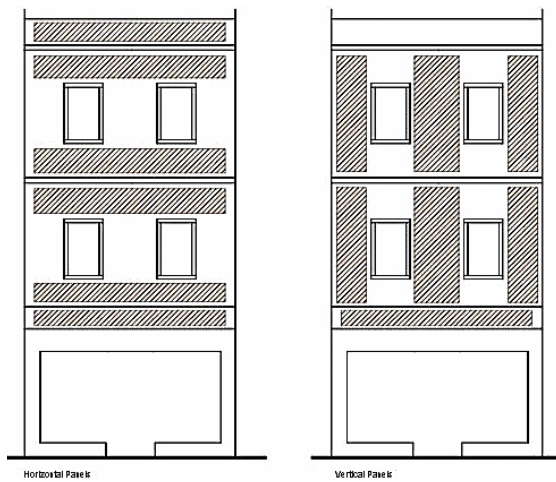
Figure 3: Sign Placements using Grid Analysis
