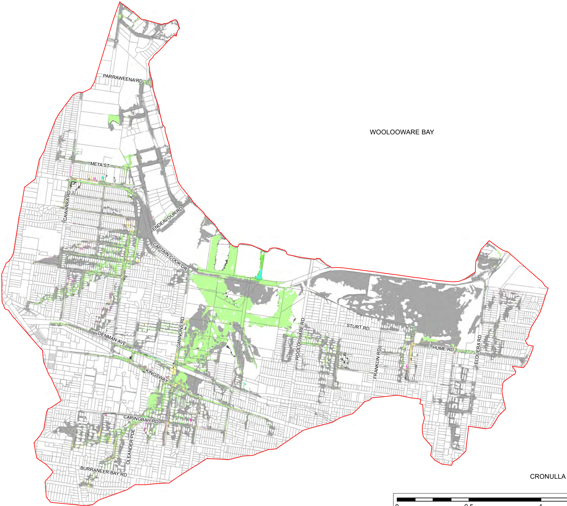
FIGURE C19 WOOLOOWARE BAY CATCHMENT CHANGE IN PEAK FLOOD LEVEL HYDRAULIC ROUGHNESS -20% 1% AEP EVENT, AR&R2019
