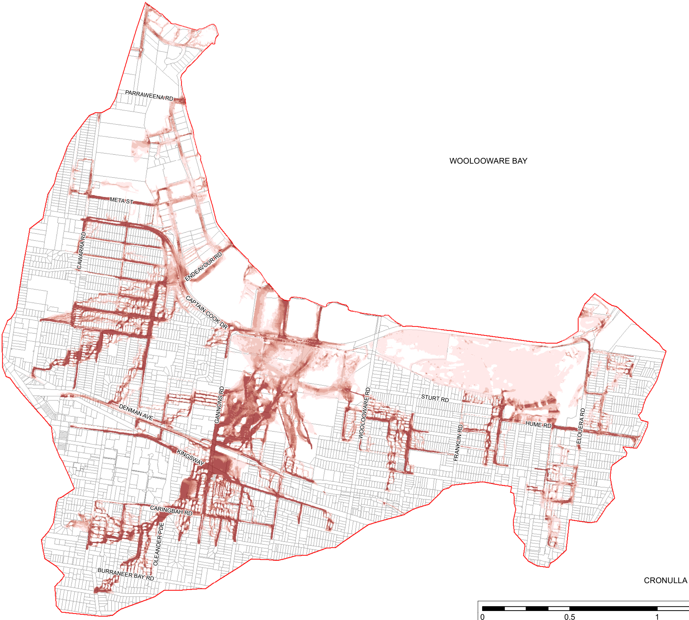
FIGURE B11 WOOLOOWARE BAY CATCHMENT PEAK FLOOD VELOCITY 0.2% AEP EVENT 2019 AR&R
