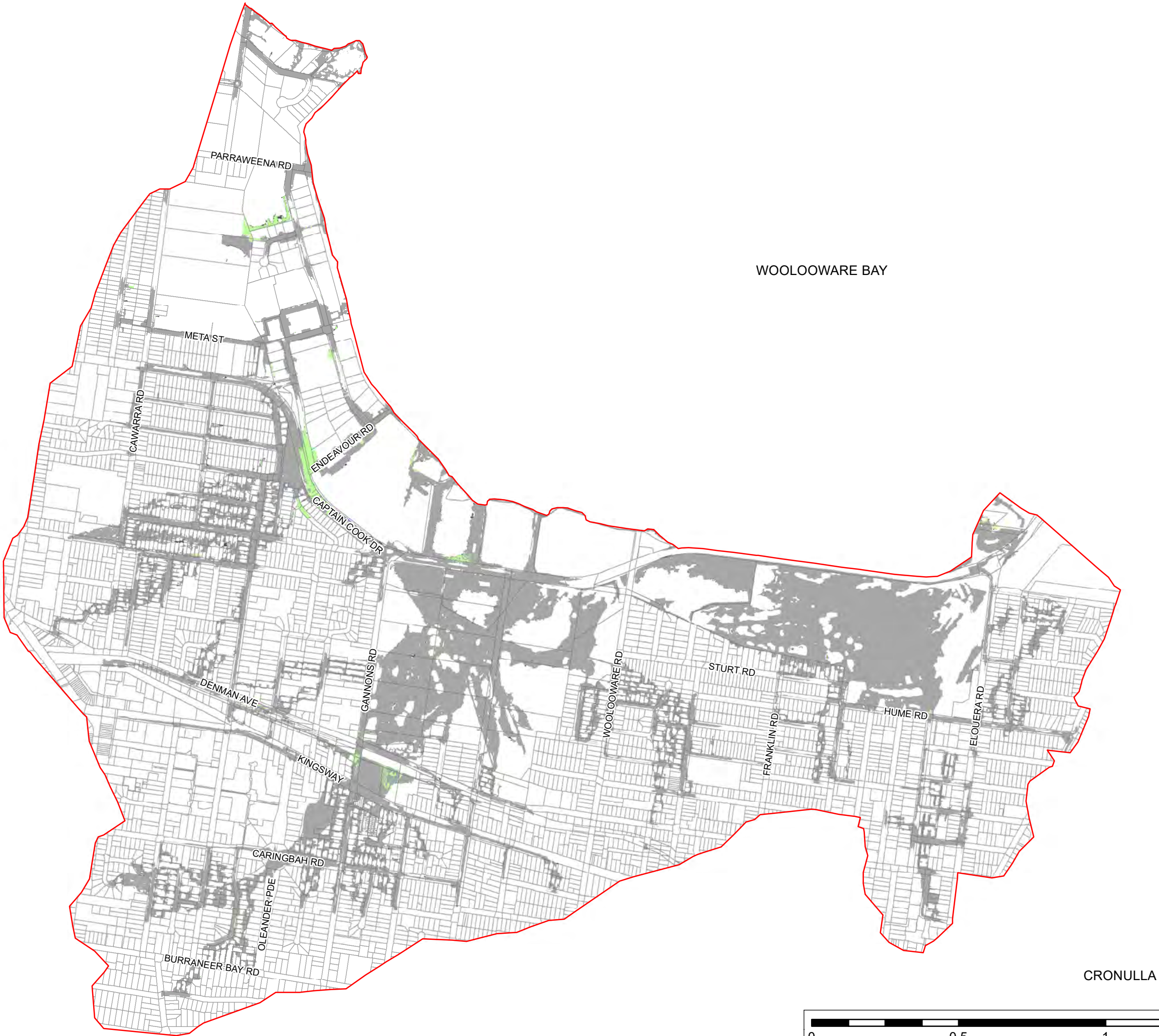
FIGURE C12 WOOLOOWARE BAY CATCHMENT CHANGE IN PEAK FLOOD LEVEL RAINFALL LOSS +50% 5% AEP EVENT, AR&R2019
