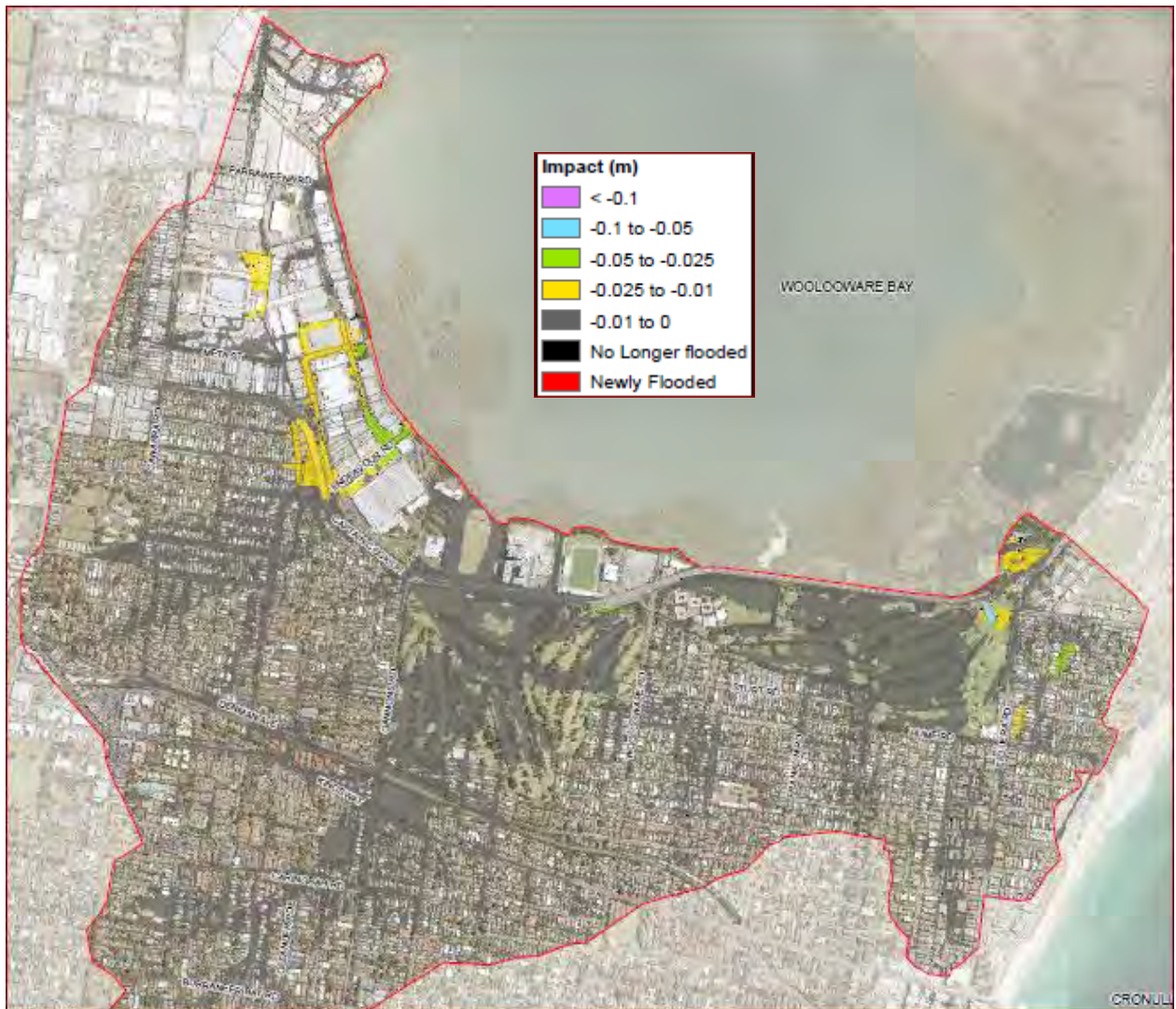
Image B2: Comparison of Enveloped 30, 120 and 540 minute durations v Envelope of all Durations
