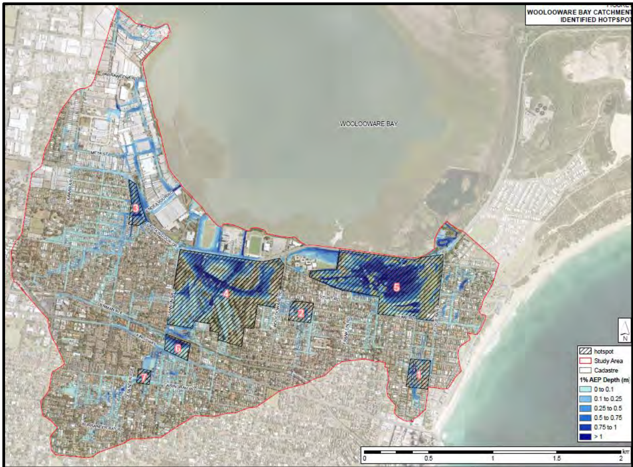
Photo 2: 1% AEP Flood Extent, Depth and Identified Hotspots
