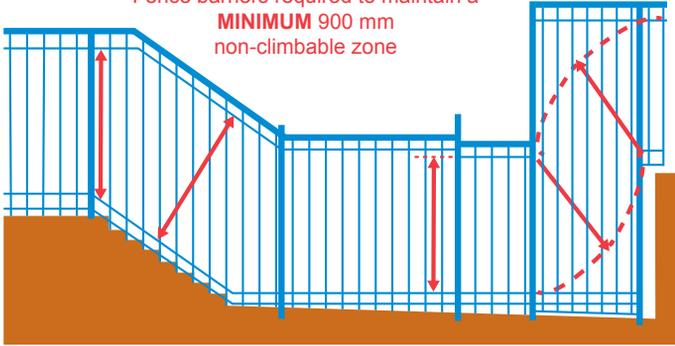
Where a barrier is sloping the measurements are perpendicular to the top of the barrier to maintain the integrity of the required NCZ and barrier height.
