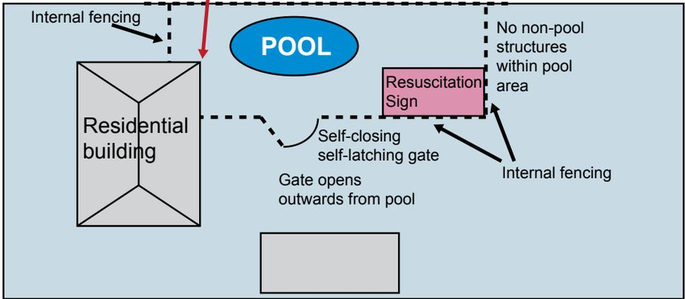
Buildings not associated with the pool, such as garage, carport, shed, boatshed, pergola clothesline or the like, are to be separated from the pool ie. outside the enclosed pool area child-resistant barriers. See diagram below..
